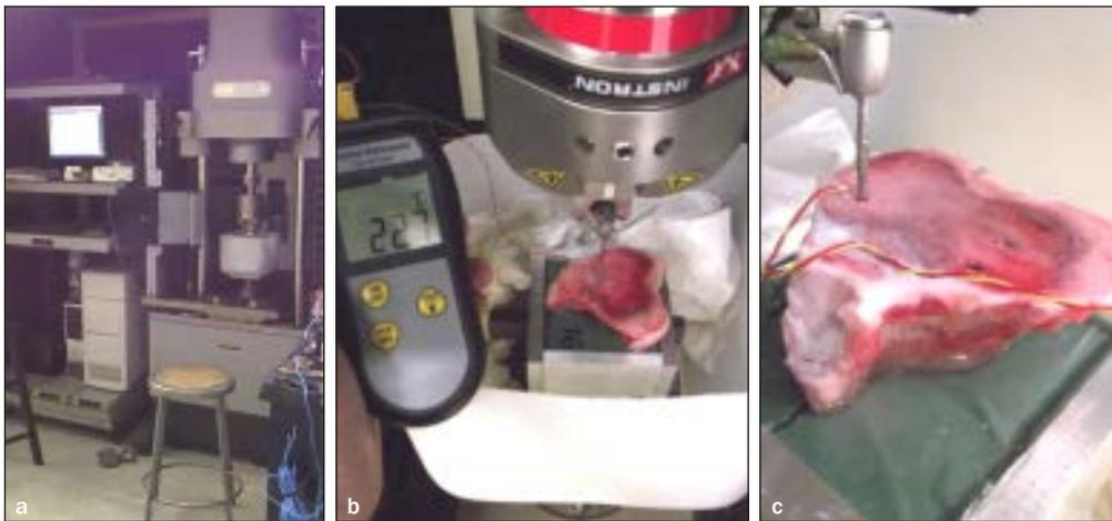
**Fig 2** (a) Materials testing machine setup. (b) Potted bone sample and drill motor installed in custom fixtures and temperature probe installed in bone adjacent to the drilling site. (c) Location and spacing of implant sites across the tibial plateau.
